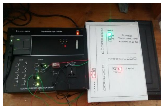
Figure 7 Model of T-Junction Traffic Control System Using a Plc
